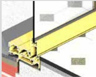
Semi and fully recessed sill options available to create seamless transition between internal and external. Semi recessed sill pictured above. Drains must be used with all fully recessed sill installations.
