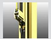
The detail above shows our heavy duty meeting rail and the recessed sash support shoe. Recessing the shoe is important, as it protects the shoe when the sash is fully opened down to the sash stop.
